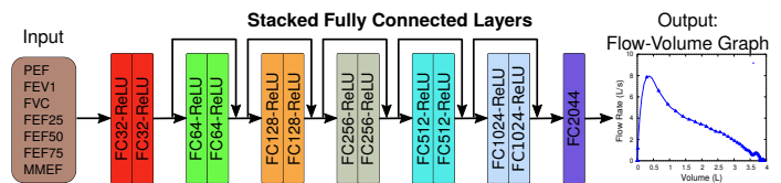
Figure 8: Deep residual decoder of the mmFlow system.
