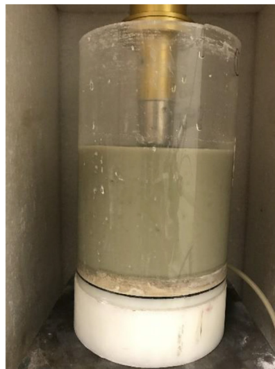
Fig. 3. Contaminated sediment treatment chamber.
