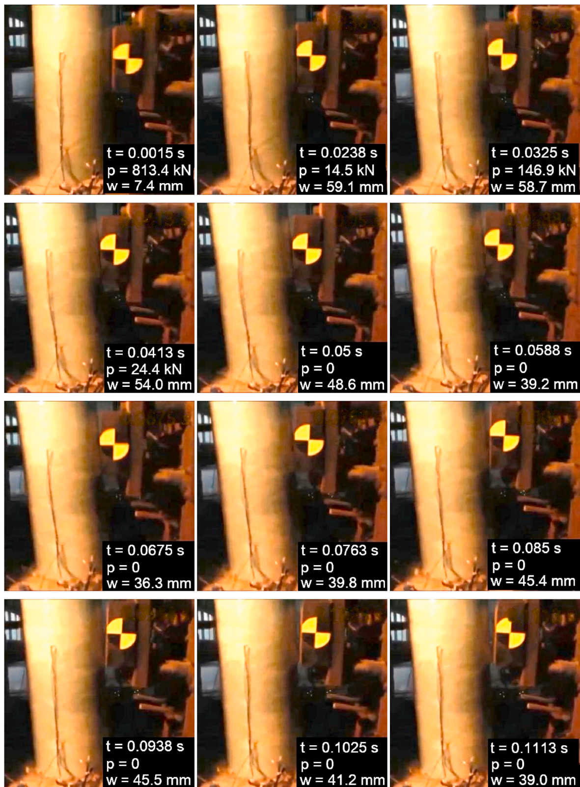
Fig. 6. Typical impact failure process (i.e. D7-II).
