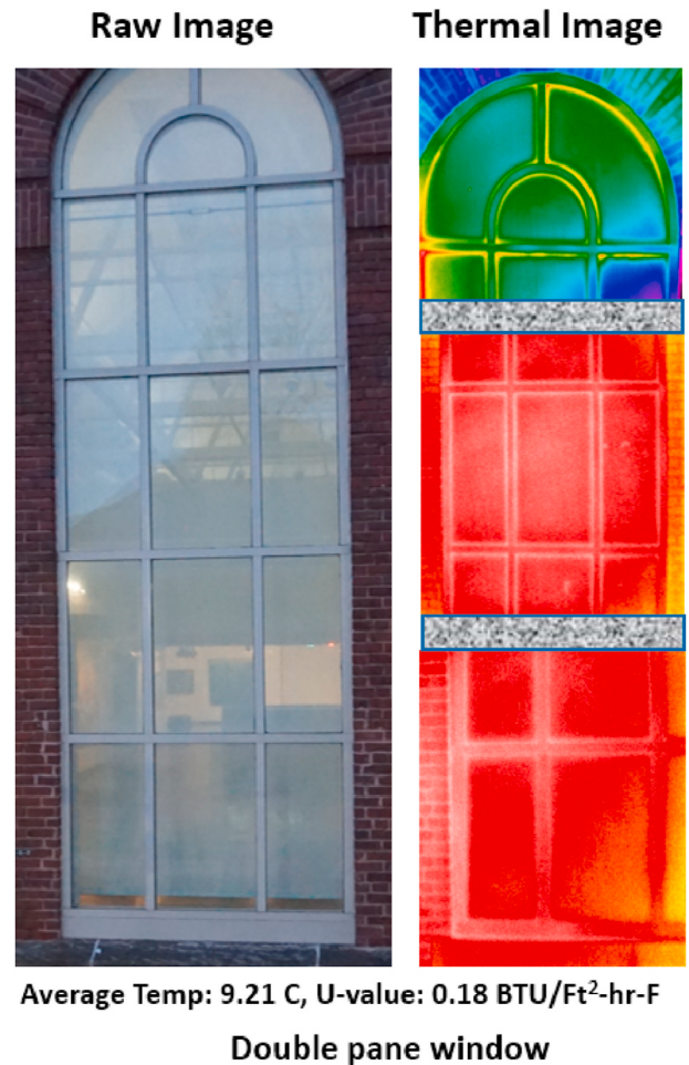
Fig. 11. Museum window 1: Double pane (temperature/U-value) captured on October 8, 2019.
