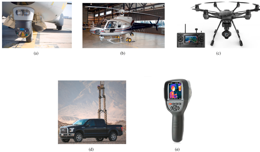
Fig. 2. Infrared thermal imagery: (a) aerial inspection using an Airbus plane [47]; (b) aerial inspection using an Airbus helicopter [48]; (c) automated fly inspection using UAVs [49]; (d) street drive inspection using vehicle [50]; (e) hand-held IR camera used for general walk through inspection [51].
