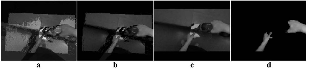
Figure 2: Aligning I_{lwir}^{raw} into the I_{rgb} with depth maps. First, (a) I_{lwir}^{raw} and I_{rgb} are overlapped onto the depth maps. (b) Next, the projected I_{lwir}^{raw} is bounded by hand temperature to capture possible hand regions. (c) Then, the projected I_{rgb} and I_{lwir}^{raw} are transformed on the RGB plane. (d) Finally, hands are cropped from backgrounds. For visualization, I_{lwir} is color mapped by a high value as red and a low value as blue.
