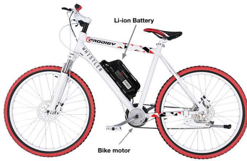
Figure 1: An electric bike is powered using an electric motor and a battery [27].
