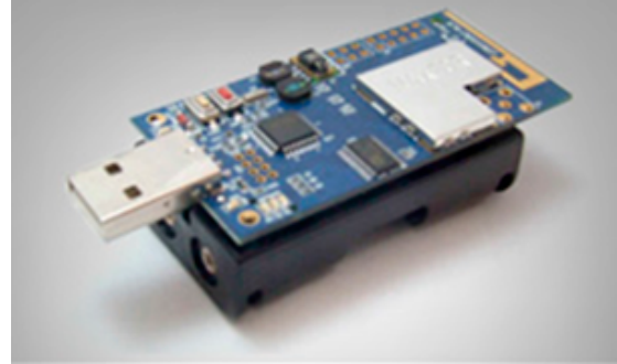
Fig. 2. The TelosB mote [13].
