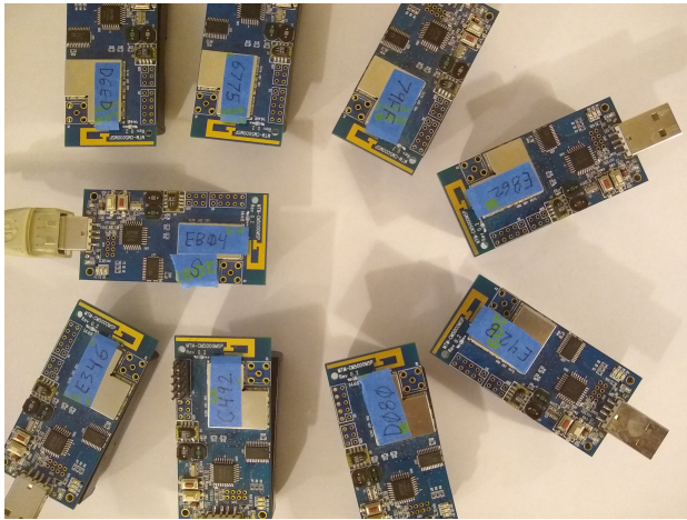
Fig. 6. Implementation setup with single server and eight clients.
