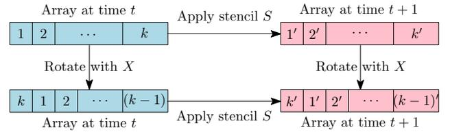
**Figure 3: The stencil  $S$  does not care where cells are with respect to the start of the array; it only cares about where they are with respect to one another. The shift matrix  $X$  does not affect cells' relative locations, so it does not change the values of the updated cells.**
