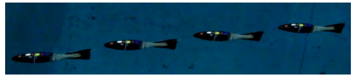
FIGURE 5. Multiple time instances from video of the robotic fish swimming in a large water tank with still water
