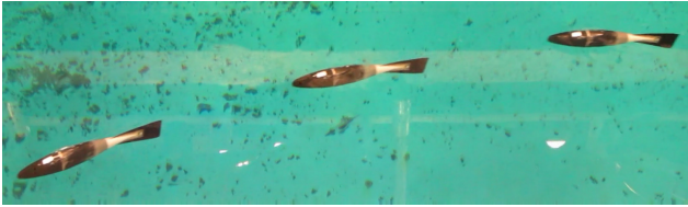
Figure 7: Time instances of the robotic fish swimming in a large water tank with a demonstration of maneuvering via combination of bursts of AC actuation and gliding with DC actuation.
