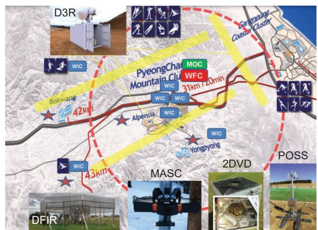
FIGURE 15. ICE-POP 2018 in South Korea, with a magnified picture of the Olympics venues, spread between the coastal area and the mountains. Some instruments at the main Mayhills supersite are shown (see the similarity with Figure 1) as well as NASA's dual-polarization, dual-wavelength ( K_u , K_a )-band radar (D3R) [25].
