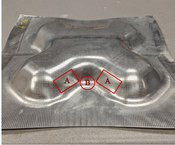
Figure 6. A demonstration part of AA7075-T6 Alclad sheet, originally measuring 470×470×1.6 mm, is shown. The white dots etched onto the surface of the demonstration part prior to forming were used to measure local major and minor strains and calculate through-thickness strain using image analysis techniques. Two locations of interest are the inner side-walls, located by red rectangles labelled A, and the inner corner, located by a red circle labelled B.
