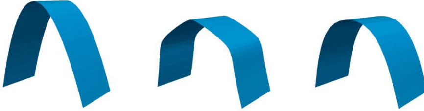
Fig. 3. Deformed plate for the cylinder metric with two modes. Left: BC PP; middle: Metric PP; right: Final. Compare with Fig. 2 corresponding to the metric (77) (one mode).
