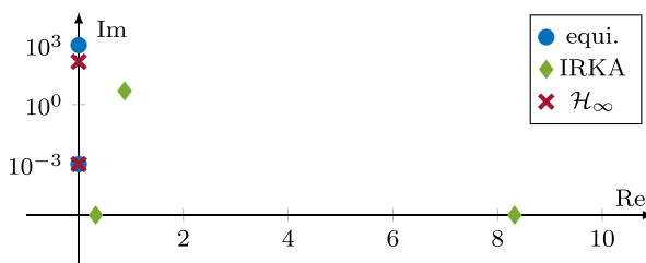
Fig. 1 Computed interpolation points for structured interpolation of the first subsystem transfer function for the time-delay system (points appear in conjugates pairs, only top half of the complex plane is depicted)
