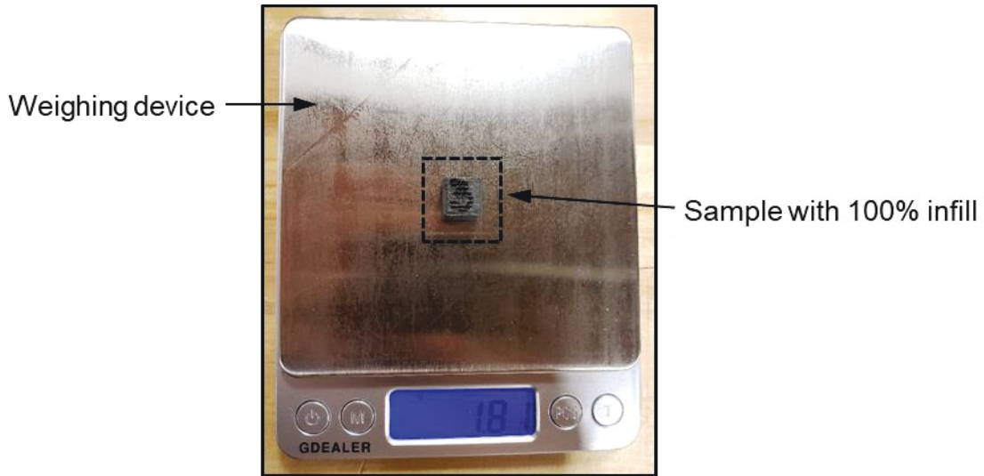
Fig.6 Weighing device measuring the sample with 100% infill
