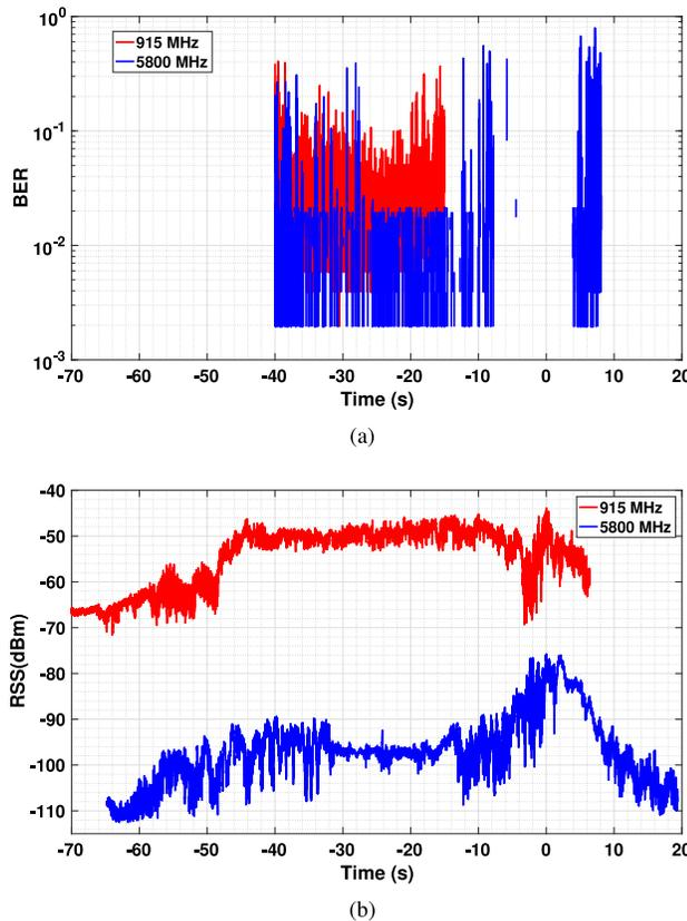
Fig. 14. Test results of V2I communication test at 915 MHz and 5.8 GHz on single receive antenna: (a) BER (b) RSS. Route from south to north. Time 0s marks the moment the vehicle passing by the road light pole of the receiver antenna.
