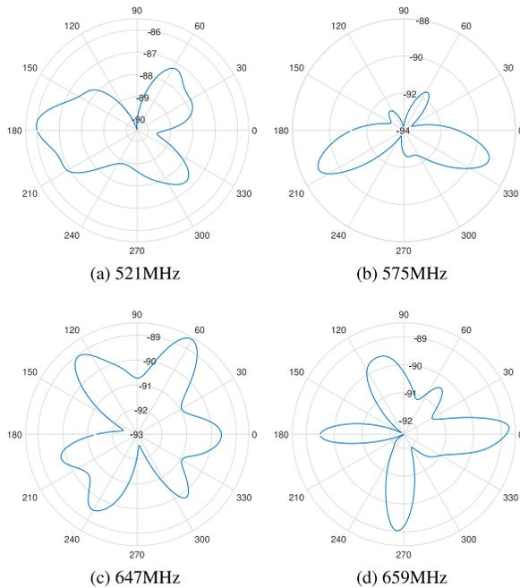
Fig. 10. Receive beamforming on  $2 \times 2$  uniform rectangular array, H-plane scan of 4 local TV channels with 6 MHz bandwidth, polar axis unit: dBm.
