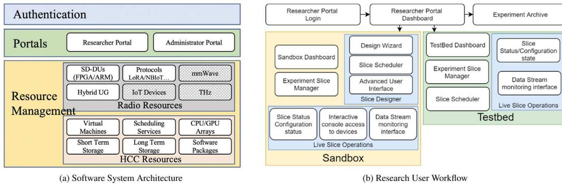
Fig. 2. CoSeC-RAN testbed software and workflow. The shaded blocks in (a) are components to be added in the near future.
