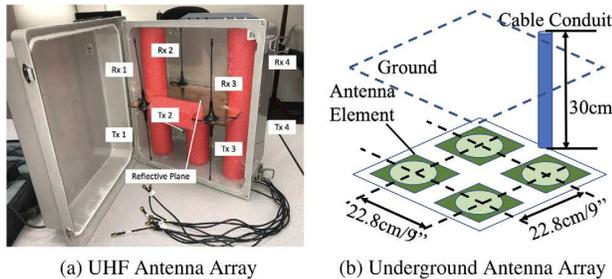
Fig. 4. UHF Antenna array:  $2 \times 2$  uniform rectangular array.
