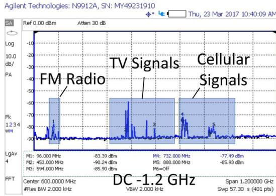
Fig. 9. Receiving spectrum of UHF antenna element in DC-1.2 GHz.
