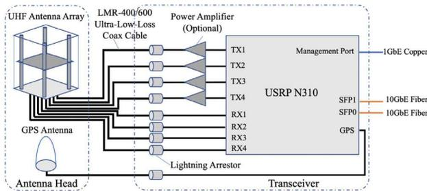
Fig. 3. Software defined distribution unit schematic.
