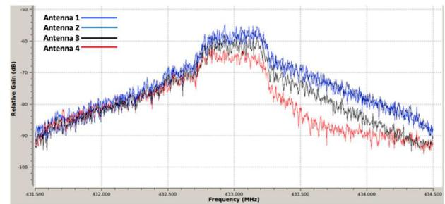
Fig. 12. The Spectrum of received OFDM signal on 4 antennas in underground to aboveground communication test.
