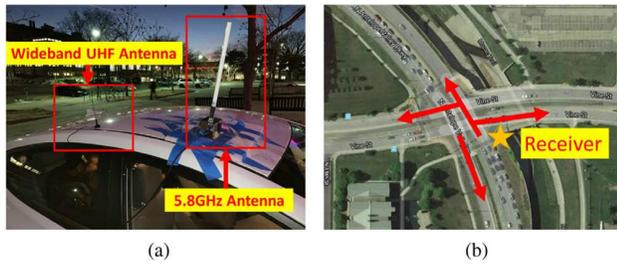
Fig. 13. V2I communication test setup: (a) vehicular antennas (b) test routes.
