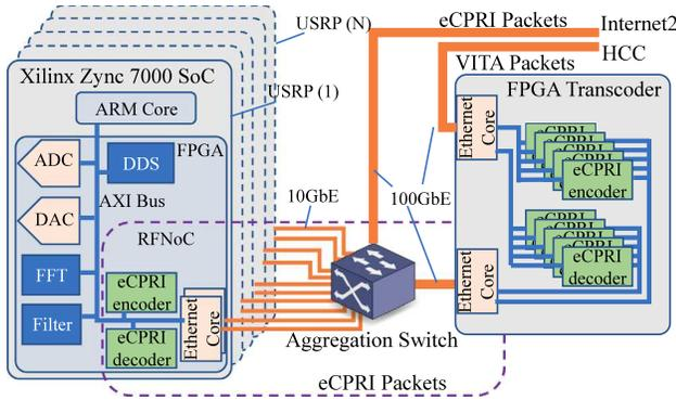
Fig. 6. The schematic of fronthaul logical for eCPRI.
