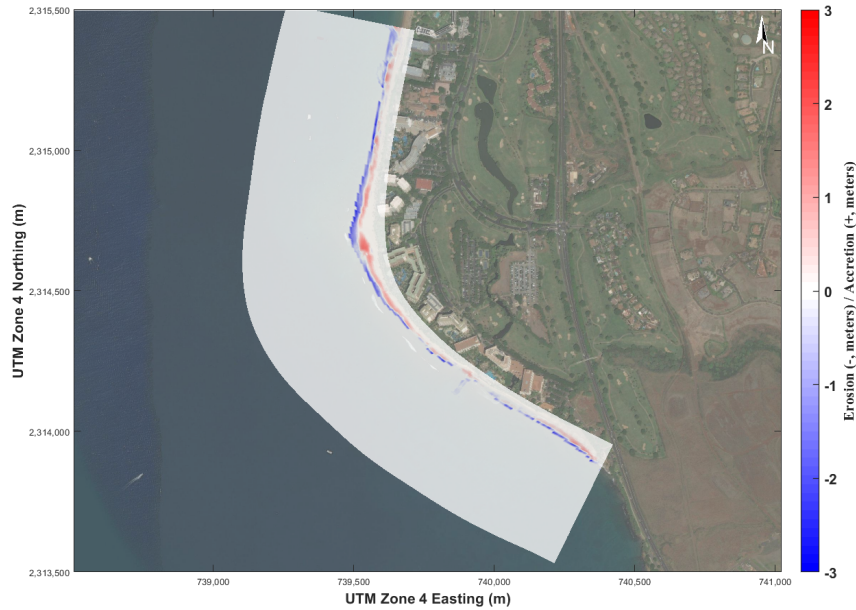
Fig. 13. Modeled sediment accretion and erosion in HLC at Ka'anapali Beach between November 1, 2015 to February 1, 2016.
