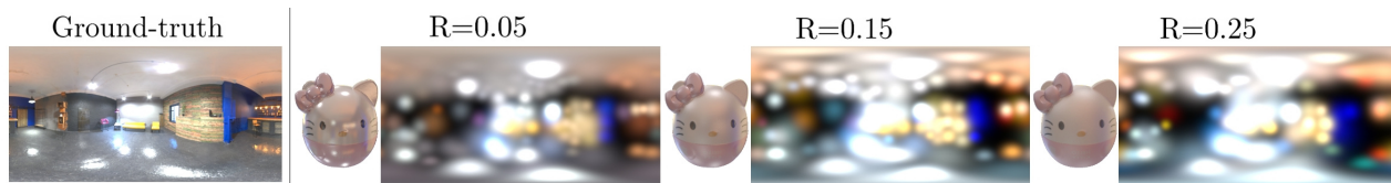
Figure 6: Ground truth and our reconstructed environment maps for the synthetic Kitty data with varying Ward BRDF roughness R . For each roughness setting, an example training image rendered by Mitsuba [14] is also shown. For rough surfaces ( R=0.25 ), PhysSG still recovers an environment map that resembles the ground truth, though blurrier. Nonetheless, this is sufficient to reconstruct the material accurately.
