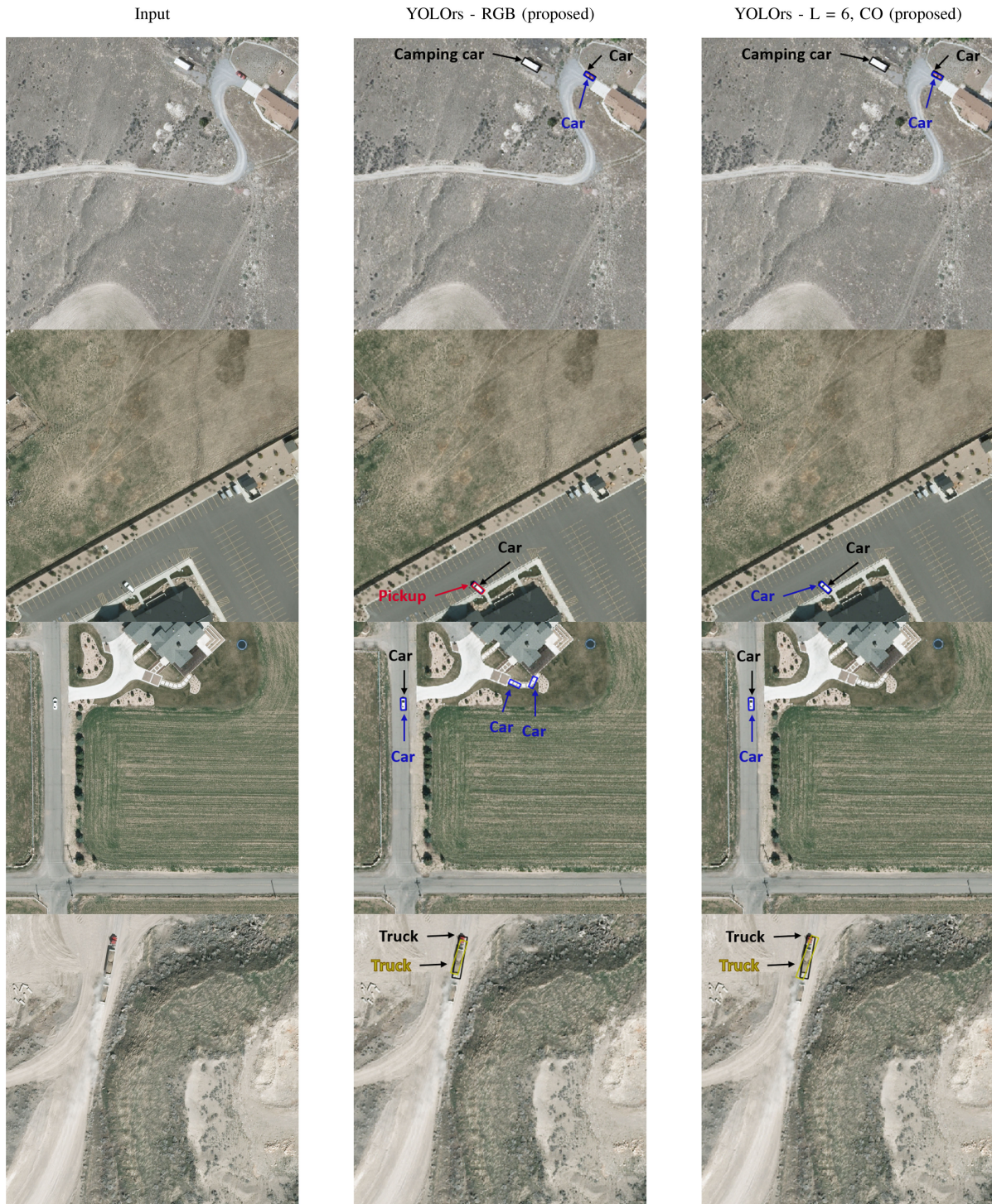
Fig. 11. Object detection using various networks. Column 1 shows the input images, columns 2 and 3 shows detections obtained by the proposed YOLOrs network in baseline RGB and fusion at layer 6 via CO configurations, respectively. Black bounding boxes and labels show the ground truth, whereas colored bounding boxes and labels show the detected objects.
