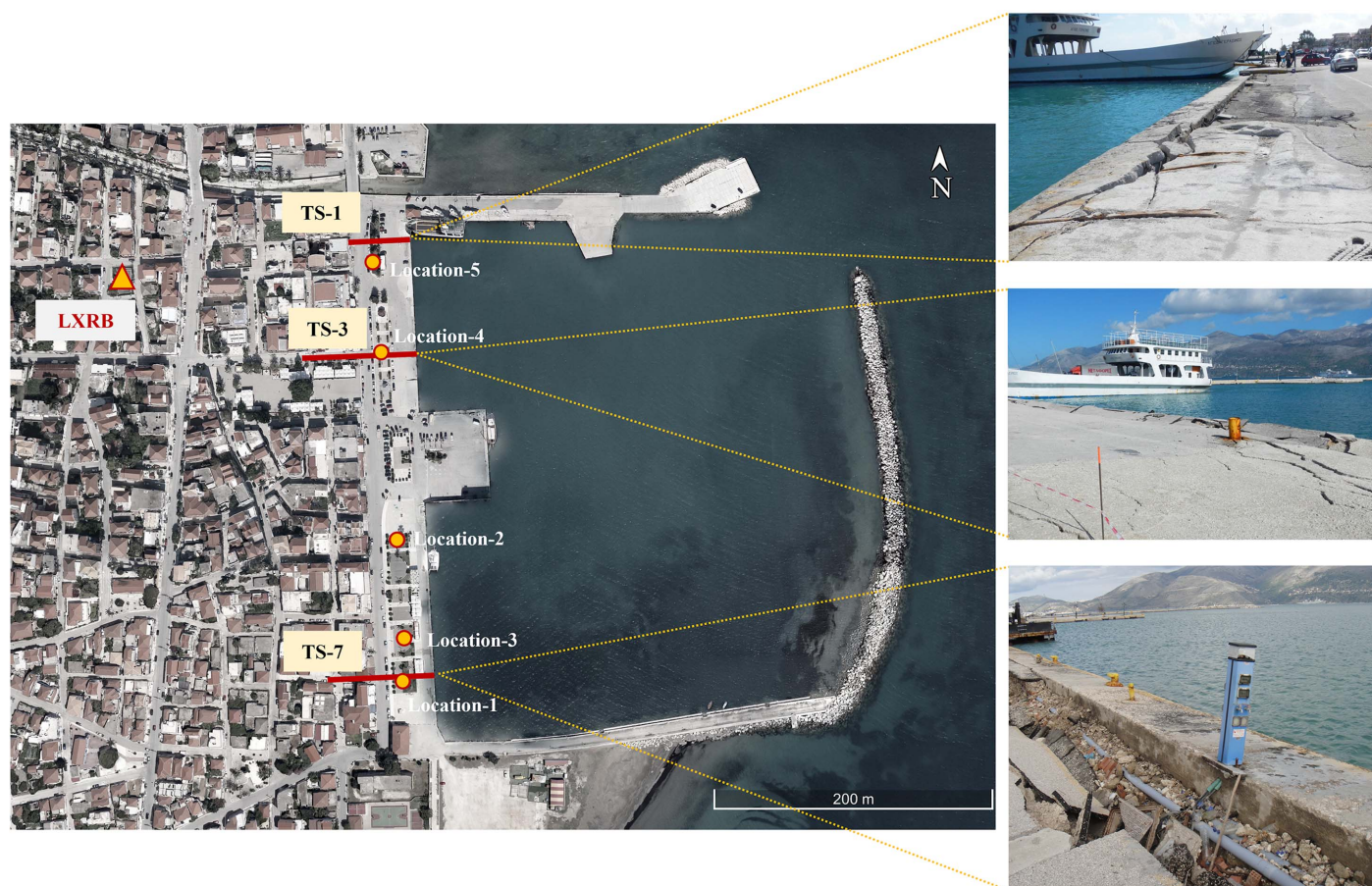
Fig. 3. Location of strong motion station, selected transects, and site investigation locations at Lixouri port, and observed quay wall damage. (Images by authors.)
