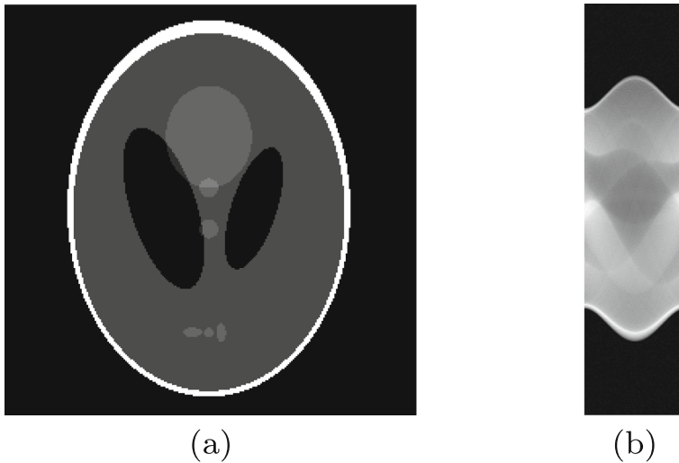
Fig. 2 Tomography test case: a True phantom ( 256 \times 256 pixels), b sinogram (90 equispaced angles in [0, \pi] , 362 measurements per angle, and 1% white Gaussian noise)
