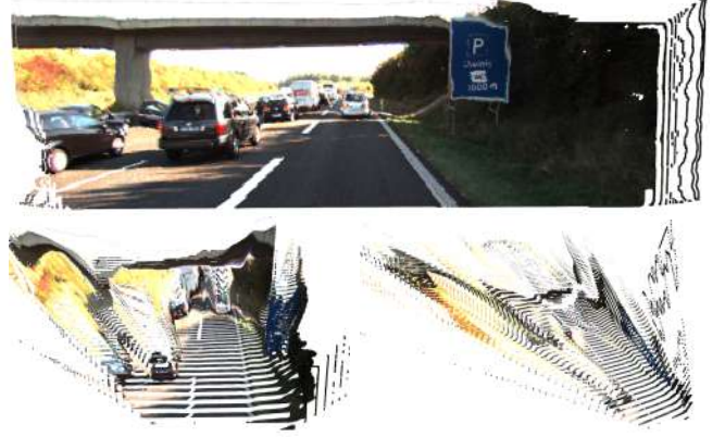
Fig. 3: Top: Front view pseudo point cloud of an image from the KITTI dataset; Bottom: Arbitrary views of the same point cloud; The point cloud is generated from the depth images estimated using a monocular depth extraction technique [38].
