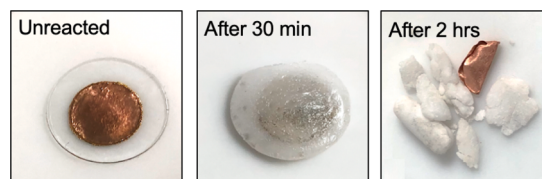
Fig. 3. Photos of model Printed Circuit Board samples before and after the pre-treatment with scCO 2 and H 2 SO 4 .
