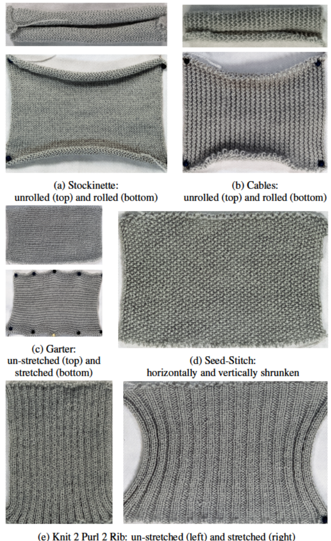
Figure 1: Exemplar textures produced during the described scenario that are curly (a), cabled (b), vertically-elastic (c), shrunk (d), and horizontally-elastic (e).
