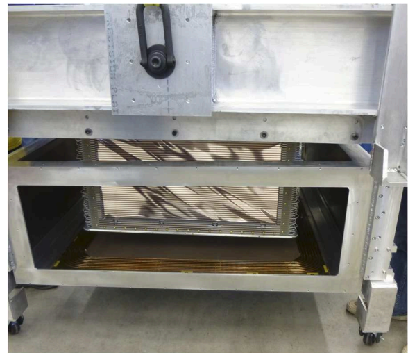
FIG. 14. Motion chassis attached to the enclosure, allowing the TPC to be supported and rotated.
