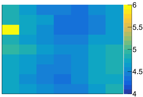
FIG. 18. Typical noise level of pads within the unit cell, with noise level in ADC channels. The orientation of the pads matches that of Fig. 7.
