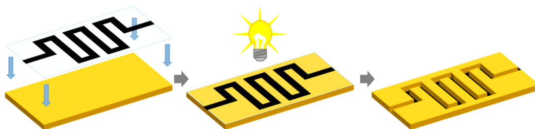
Figure 84. General procedure for photomasked image transfer for microfluidic device fabrication. A mask is placed over monomer mixture and exposed to light. Masked regions form channels and other negative features in the generated device.
