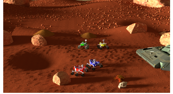
Fig. 3: The 3D visualization of the modified rover domain. There are four robots on Mars, each has a different camera resolution and sampling equipment. The mission is to sample soil, rock and take images at different locations and communicate it to the lander shown on the right side of the picture.
