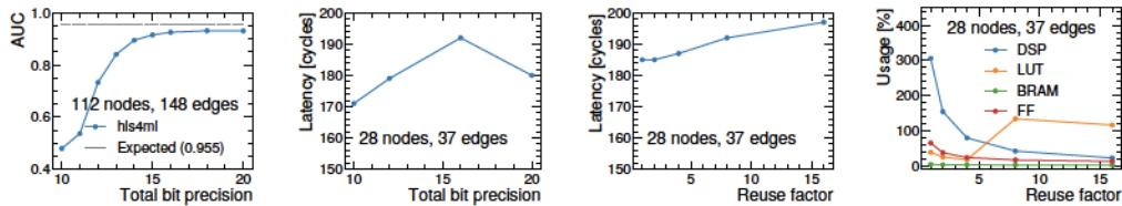
Figure 4: Alternative GNN segment classifier model implemented in `hls4ml`. AUC (far left) and latency (center left) in clock cycles for a 5 ns clock period as a function of the total bit width. The reuse factor (and thus II) is set to be 8. Latency (center right) and resource usage estimates (far right) relative to the available resources on a Xilinx KU 115 FPGA versus reuse factor for fixed total bit precision  $\langle 16, 6 \rangle$ .
