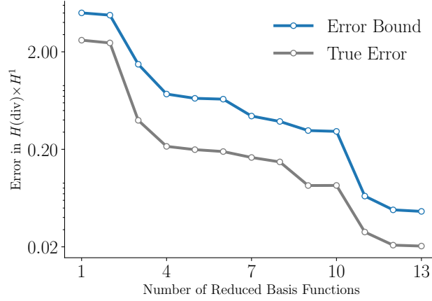
Fig. 8: Convergence of the error bound and true error for increasing RB basis dimension N . The parameter value is \mu \approx (.223, .244, .746) , corresponding to the largest over-estimation of the error.
