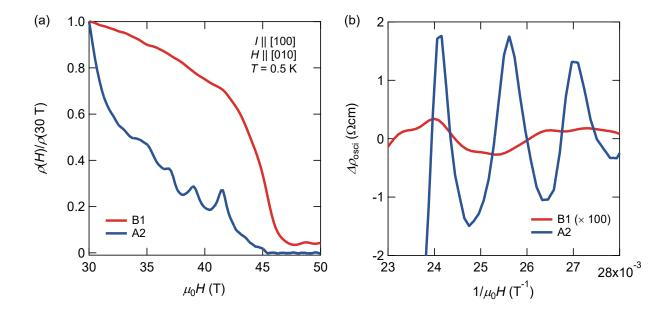
FIG. 4. (a) Magnetoresistance normalized by the resistivity at 30 T,  $\rho(H)/\rho(30 \text{ T})$ , measured at 0.5 K for B1 microstructure (red) and A2 single crystal (blue). (b) The oscillatory part of the magnetoresistance  $\Delta \rho_{\rm osci}$  obtained by subtracting a polynominal background from  $\rho(H)$ .
