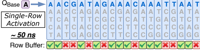
Fig. 5: K-mer matching in Sieve using Single-Row Activation and vertical data layout.
