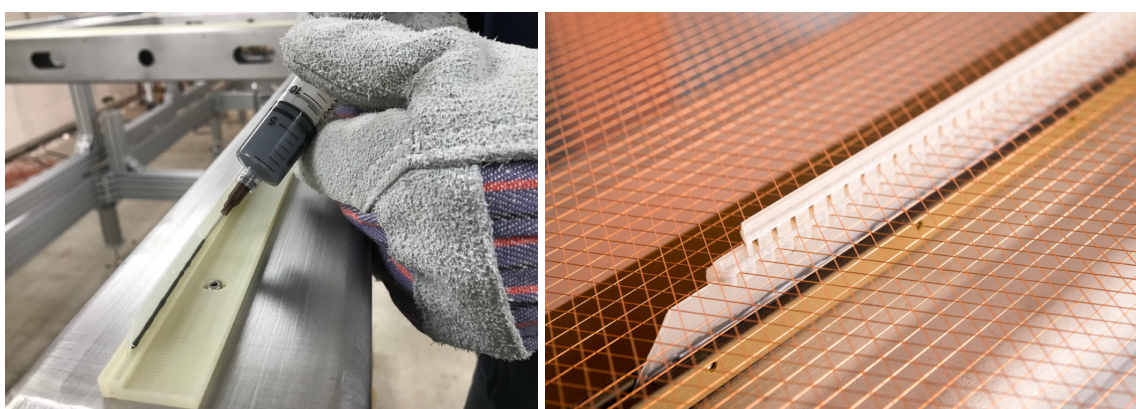
Figure 18. Left: the adjustable base slats of the combs being epoxied in place after their level has been set. Right: a finished stack of combs encapsulating the wires.
