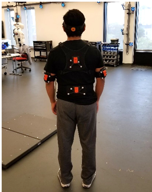
Figure 1 — Sensor configuration showing Xsens inertial measurement units (rectangular sensors on harnesses) and optical motion capture system (markers on harnesses, cameras around the room).
