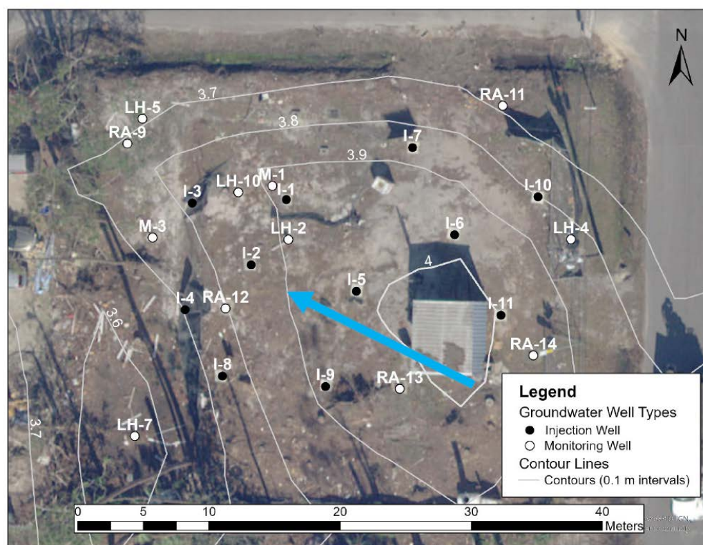
Figure 1. Aerial view of study site in northwest Florida overlaid with the groundwater elevation contour lines (0.1 m intervals), injection wells (in black), and monitoring wells (in white). Groundwater flow direction is shown by the light blue arrow. Modified from Fischer et al. [26].
