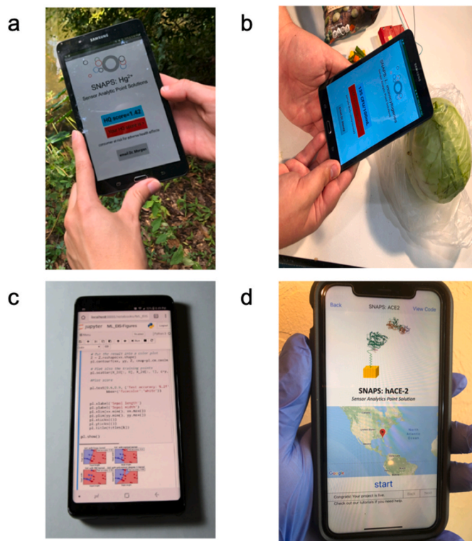
Fig. 12. Examples of SNAPS for on-site sensing with embedded data analytics and decision support. a) Electrochemical aptasensor for detection of heavy metals in drinking water; reprinted from McLamore et al. (2019) with permission from © MDPI. b) Impedimetric aptasensor for measuring Listeria spp. in fresh produce samples; reprinted from McLamore et al. (2019) with permission from © MDPI. c) Smartphone machine learning analytics for sample classification in small protein sensing; reprinted from Rong et al. (2018) with permission from © Royal Society of Chemistry. d) Impedimetric biosensor for measuring SARS-CoV-2 on surfaces using the human receptor ACE-2; reprinted from Datta et al. (2020) with permission from © MIT Libraries.
