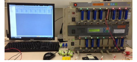
Figure 17: Neware battery tester
