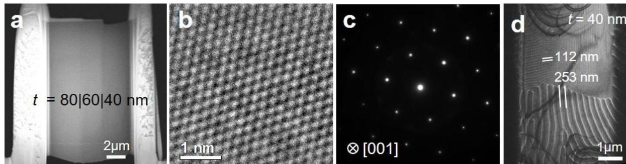
**Figure 1.** Figure 1. (a) FIB sample of Fe<sub>3</sub>Sn<sub>2</sub> with varied thickness of 40 nm, 60 nm, and 80 nm. (b) HRTEM image and (c) SAED pattern of Fe<sub>3</sub>Sn<sub>2</sub> sample. (d) Lorentz TEM image of 40 nm thick Fe<sub>3</sub>Sn<sub>2</sub> showing the stripe domain structures with different domain widths.
