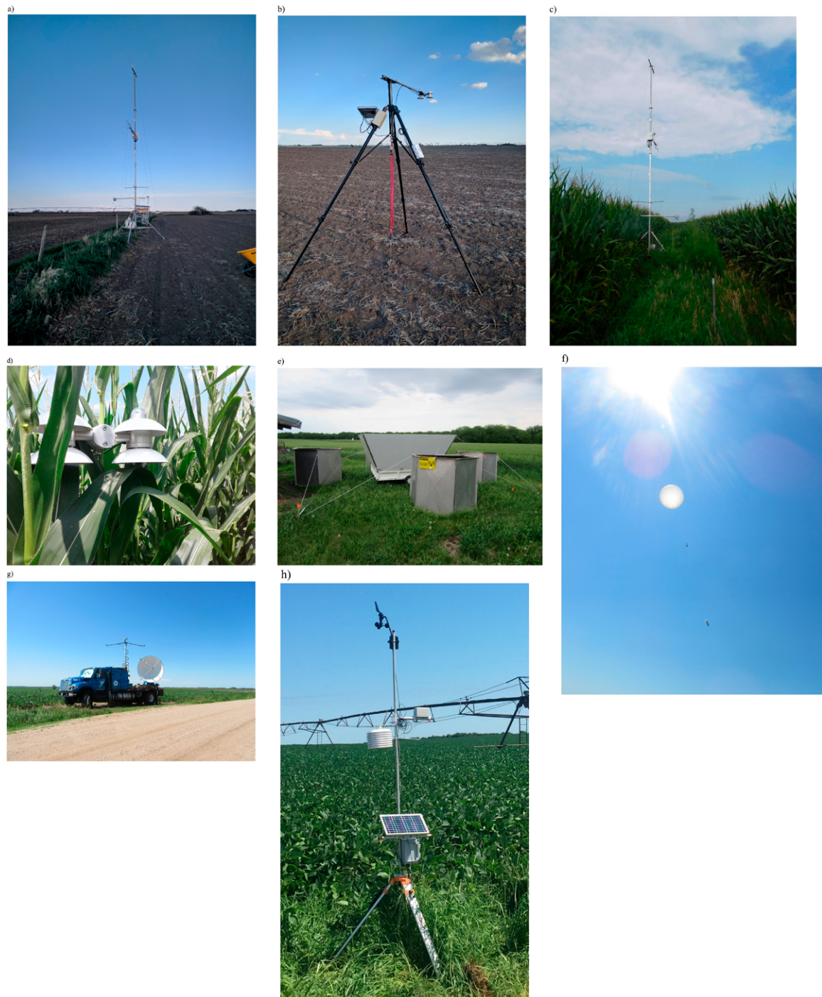
Fig. 2. (a) An irrigated ISFS tower (site 1 in Fig. 1) at the beginning of the IPO1 with a center-pivot irrigation system in the background, (b) a tripod with net radiometer during IOP1, (c) same ISFS tower but for IOP2 (middle of the growing season), (d) net radiometer during IOP2 (middle of the growing season), (e) ISS radar wind profiler, (f) a launched radiosonde balloon, (g) one of the three Doppler on Wheels (DOW), and (h) an EMESH station next to an irrigated field.
