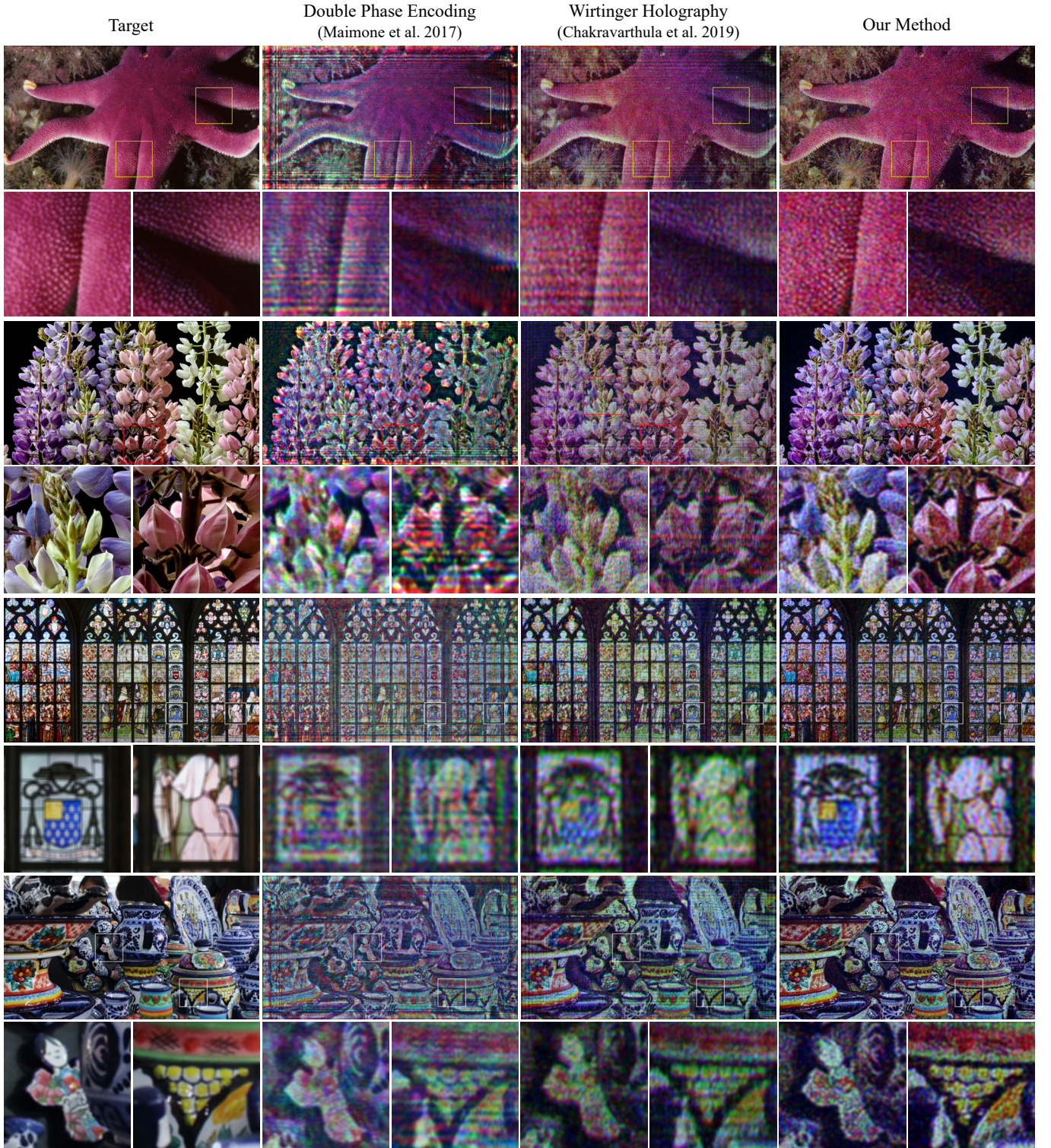
Fig. 8. Experimental Validation. We computed aberration compensated phase holograms using the proposed hardware-in-the-loop approach. We captured RGB color images of these aberration compensated holograms in a color sequential manner. The same camera settings were used for all the image capture experiments while the output laser power was adjusted to white-balance the illumination. Note that the laser power was adjusted (increased) for double phase encoding holograms due to the unwanted loss of light in the double phase encoding approach.
