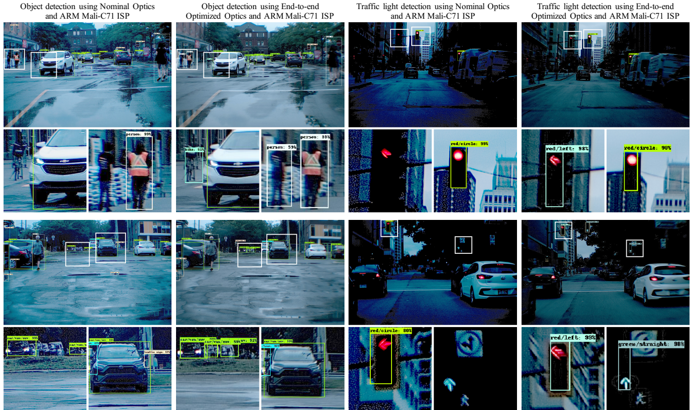
Fig. 10. Real-world prototype captures for automotive object and traffic light detection with Cooke triplet and hardware ISP. The manufactured prototypes are tested in the wild and demonstrate that our optimization allows for higher accuracy object and traffic light detection and classification. Note that our traffic light detector is trained to recognize vehicle traffic lights and ignores pedestrian traffic lights. The optimized optics have greater light efficiency (smaller f-number) and more uniform blur across the field of view than the nominal optic, which leads to greater detection performance. The optic optimized for traffic light detection is slightly sharper in the center and the peripheries than the optic optimized for object detection due to the size of traffic lights. Note that the object detection captures were taken during daytime whereas the traffic light detection captures were taken at dusk.
