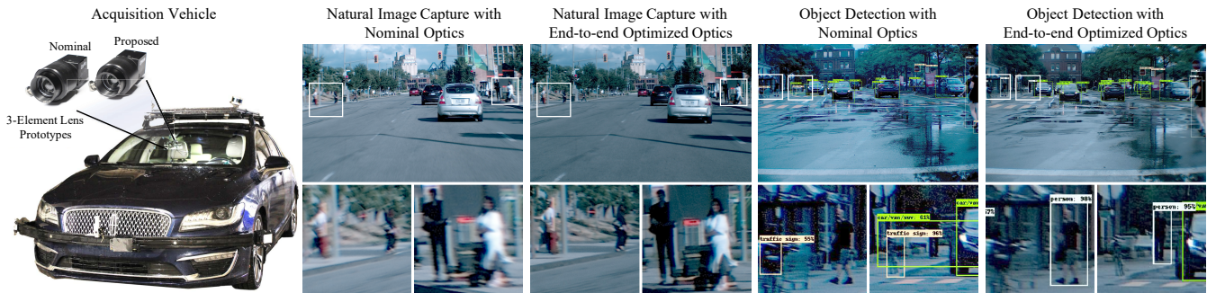
Fig. 1. We propose an end-to-end camera design scheme that jointly optimizes compound optics together with hardware and software image post-processors. Our approach allows us to cater lens systems and the hyperparameter settings of the entire imaging pipeline towards domain-specific applications, including but not limited to automotive object detection and natural image capture. We leverage existing traditional optics design tools such as Zemax, which can be easily integrated into our framework. We validate our method in simulations and in the real-world via manufactured prototypes, using an (optimized) ARM Mali-C71 ISP and cameras mounted onto an acquisition vehicle (left). When optimizing for perceptual image quality (center), the proposed method finds an optics and processing pipeline that improves visual detail across fields, outperforming conventional pipelines with a nominal lens resulting from over one month of Zemax-aided expert-design. When optimizing for a pedestrian-vehicle detection (right), the same method learns different optics with comparable spotsizes but significantly higher speed ( f/3.2 ) than the nominal optics ( f/4.4 ), improving object detections in flux-limited image regions that are challenging to recover by fine-tuned conventional imaging and detection pipelines.
