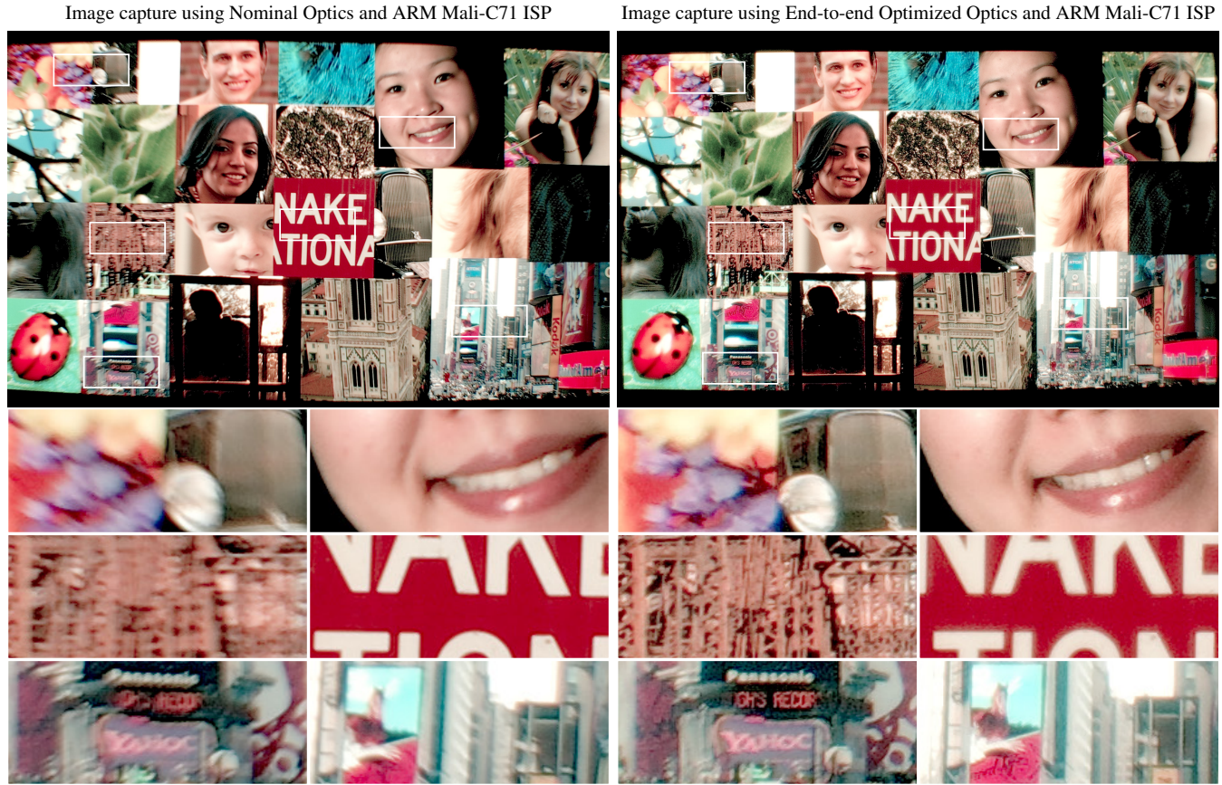
Fig. 14. Real-world prototype captures for image quality with Cooke triplet and hardware ISP. In this experimental capture we use a screen to display natural images. The image produced using the manufactured nominal optics (left) is blurrier than the image produced using our manufactured optimized optics (right). As discussed in the text, the optimized optics trades off slight defocus in the center of the scene for drastically improved image quality throughout the entire field of view. This trade off is a result of the limited degrees of freedom of the Cooke triplet and that a compound lens with greater degrees of freedom does not require this trade off as shown in Sec. 6.2. The six insets below the full image further highlights the differences. Note that since these images were captured sequentially, there is an unavoidable slight misalignment between the images captured using the two optics.
