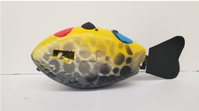
Fig. 8: Tail-actuated robotic fish used in experiments, developed by the Smart Microsystems Lab at Michigan State University. It maneuvers in water by oscillating its tail fin.
