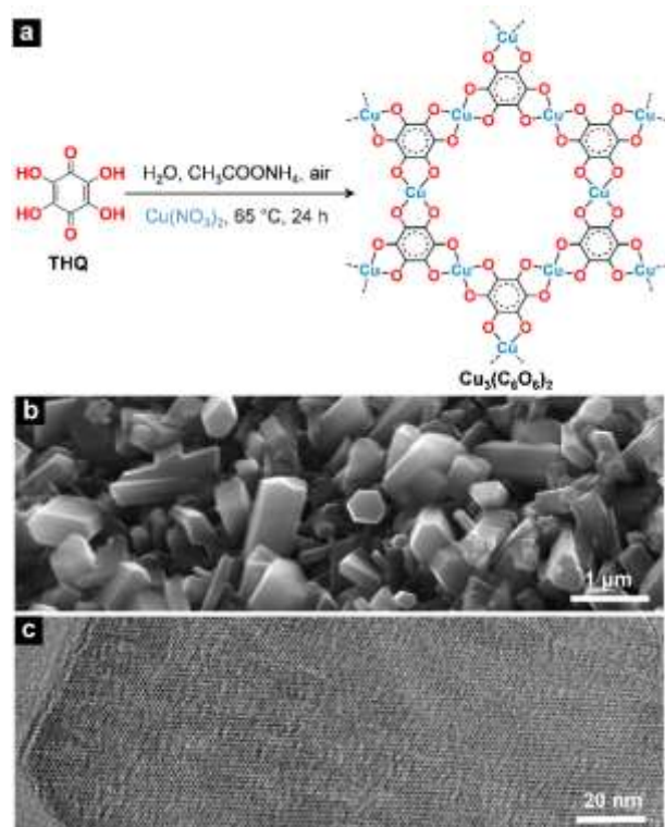
Figure 1. The synthetic scheme, chemical structure, and electron microscopy images of \text{Cu}_3(\text{C}_6\text{O}_6)_2 MOF. (a) The synthetic scheme for the formation of \text{Cu}_3(\text{C}_6\text{O}_6)_2 . (b) SEM and (c) TEM characterization of \text{Cu}_3(\text{C}_6\text{O}_6)_2 .
