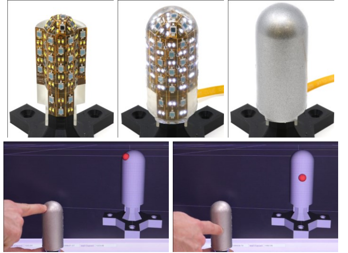
Fig. 1. A multicurved tactile finger. Top: finger through various stages of construction. We 3D-print a rigid skeleton, on which we attach a flexible circuit board with light emitters (LEDs) and receivers (photodiodes). We then mold a 7 mm thick transparent layer acting as a waveguide. Finally, we add a thin reflective outer layer. Bottom: finger performing touch localization and force detection. Location of red sphere shows predicted touch location, and sphere radius is proportional to predicted normal contact force.
