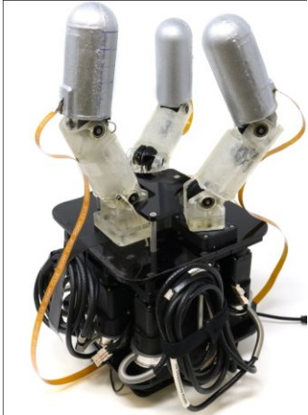
Fig. 8. A robot hand with three of the tactile fingers presented here. The palm also houses eight motors, each equipped with a torque sensor.
