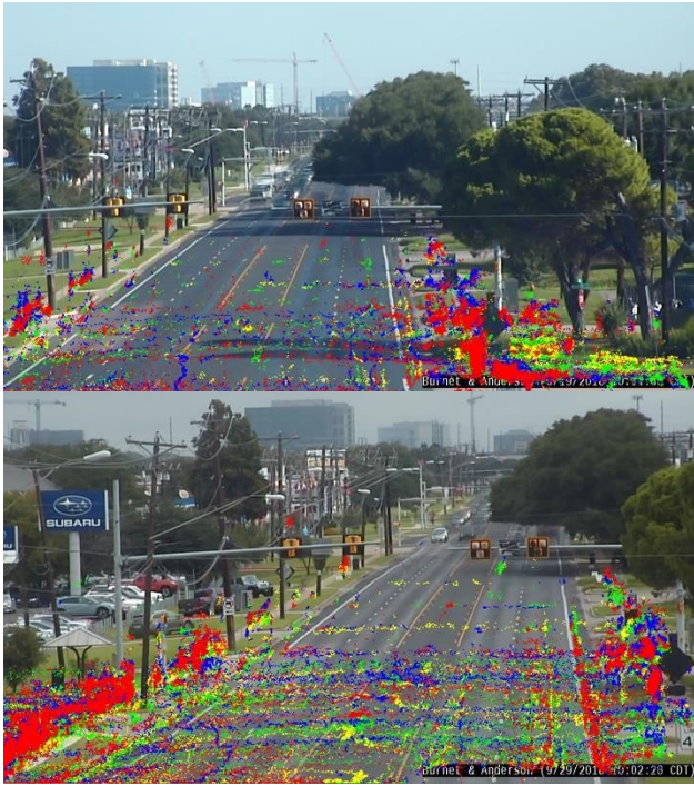
Fig. 5. Dot plot view to show locations of pedestrian activity detection before the PHB installation. The activities are colored for four time periods of the day: Yellow: 7-10 am; Green: 10:00-13:00; Blue: 13:00~16:00; Red: 16:00 ~19:00 (top) Sep 19-21 2018 (Wed ~ Fri) (bottom) Sep. 29 ~ Oct 2 2018 (Sat ~ Tue)
