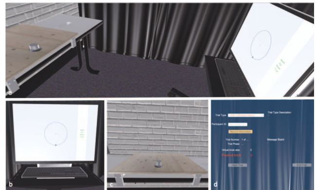
Figure 5: Virtual models developed for the study a) Virtual experimental room replicating the real environment. b) Reporting screen replicating a Microsoft Surface Studio machine. c) Tracking table, d) Researcher GUI.
