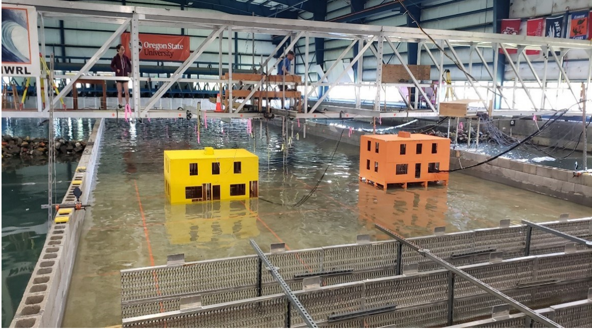
Figure 3. Photo of the directional wave basin after Trial 3. On-grade specimen (left) shows damage from previous trials.
