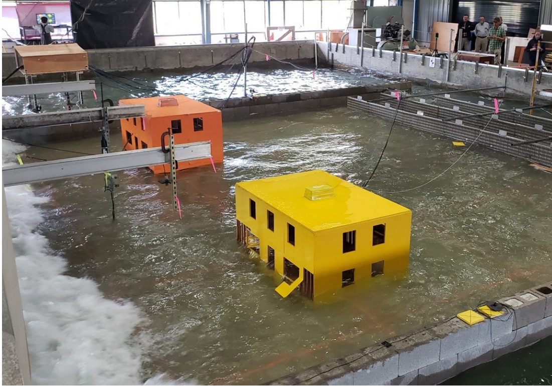
Figure 11. Photo taken during trial 10 ( h_0 = 1.30 m) that shows the damages the specimens experienced during testing.
