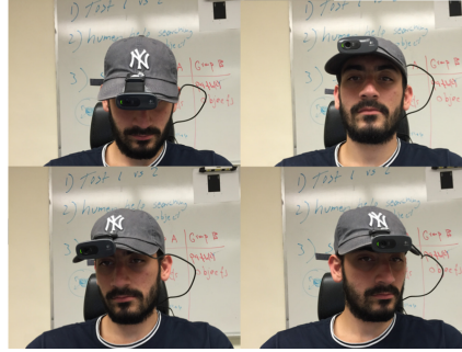
Fig. 5. The head poses giving maximum speed in different directions when continuous control is activated. The same poses correspond to the discrete commands when discrete control is evaluated in the first user study. Commands for forward, backward, right, and left are shown from top left to bottom right in clockwise order.
