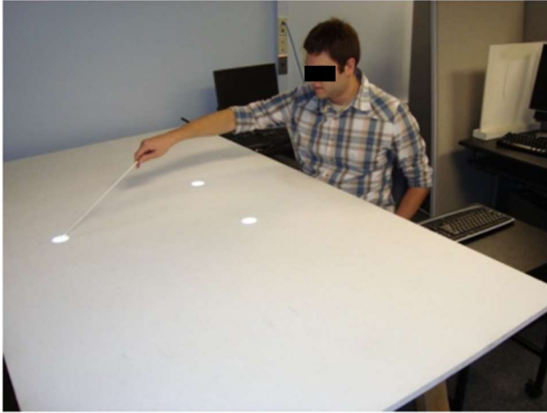
Figure 1. Experimental set-up for experiments on tool use and perceived shape (left panel). The participant estimated triangle shape by manipulating the shape of the triangle on the monitor to their right, then reached for the far circle with or without the tool. The hypothesized effect of seeing the target as closer (dotted circle) on perceived triangle shape (dashed lines) is to make the triangle appear squatter (right panel).
