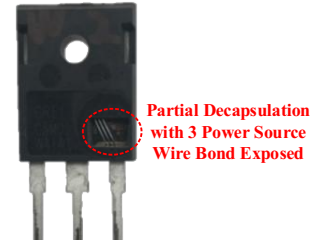
Fig. 2. New device with de-capsulation on the source-pin area.
