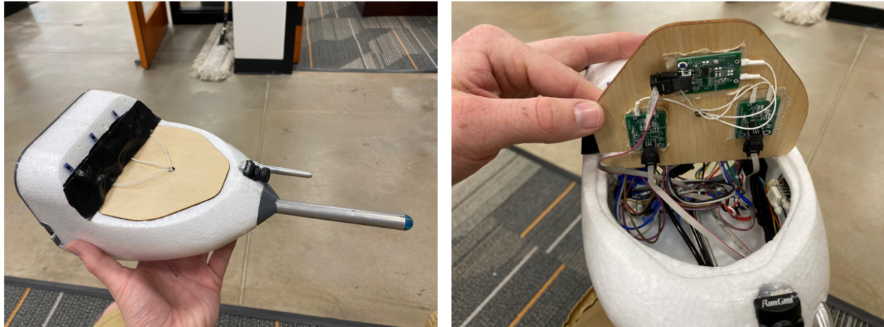
Fig. 3 Installation of prototype sensor package in Nimbus nose.
